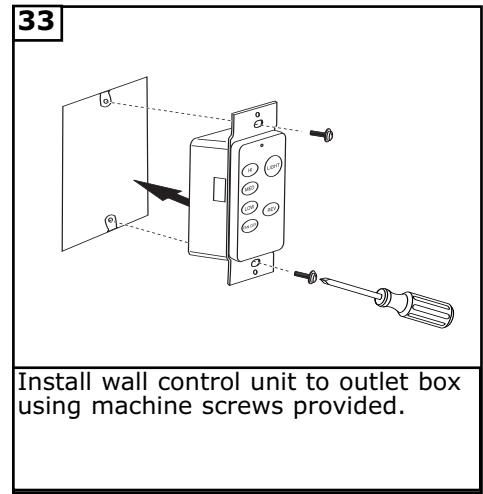
33 Install wall control unit to outlet box using machine screws provided.
